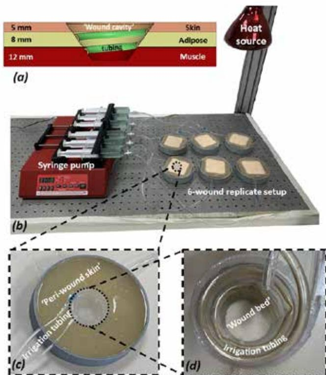
Figure 1. The experimental setup and its components
