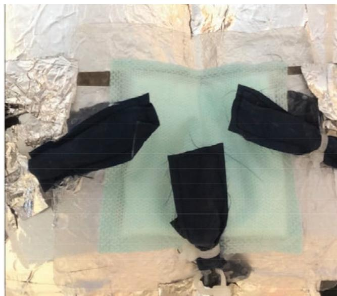
covered all three sensors. Sensors placed outside the dressing lined up with those under the dressing (Figure 4). The indenter was lowered so that it settled on the support surface and transferred the full load of 64lbs  $\pm$  2.25lbs (just over 29kgs  $\pm$  just over 1kg) to the support surface. A seventh sensor was used to measure ambient temperature and humidity. An EK-H4 Viewer program was set to log data at 30-second intervals through the test period.
