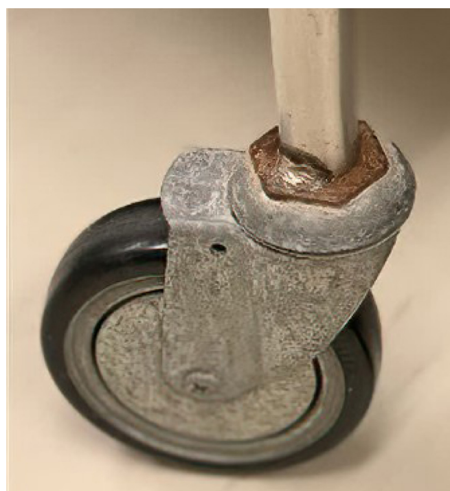
Figure 2. Rust/corrosion on galvanised forks and attachment point to WDT
